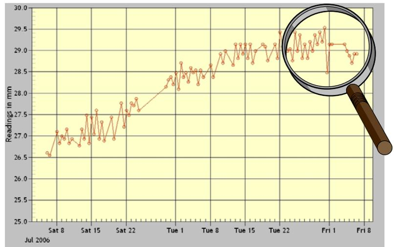
The characteristic signature of root induced clay shrinkage is plotted - left - and we have superimposed (bold black line) the electro-level plot with the dotted line representing curve fitting.
